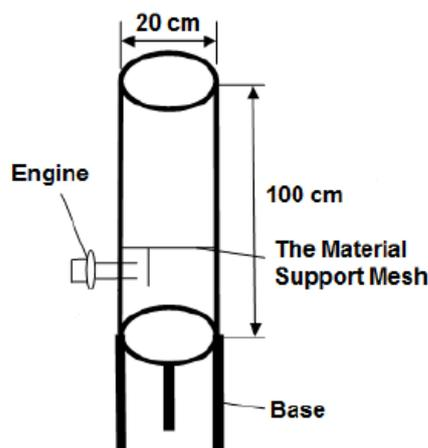
Fig. 1. Vertical pilot for co-compost schematics plot.
